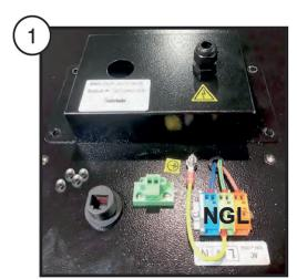
Remove the cover to get access to the electrical power block and RJ45 port.
