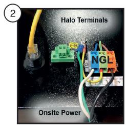
Electrical connection: Each unit must be grounded. For electrical connection, reference diagram above.
