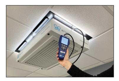
For a new filter, the measured value must be within the tolerances of the table below. If the value is higher, the filter may be incorrectly installed or have a defect.
