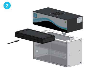
Insert the carbon filter at the bottom of the storage and place it
