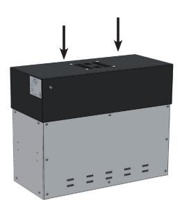
Replace the protective cover and reconnect the appliance to the mains
