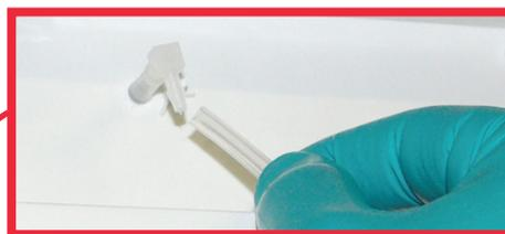
Disconnect the power supply to the fan unit followed by the fan module hose (if the device is fitted with a type A or FMolecode)
