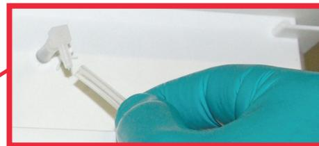
Reconnect the power supply to the fan unit and the hose to the sampling port.
