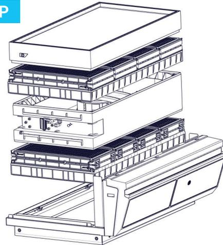
When reassembling the filtration column, be sure that the fan module is positioned correctly to access your connection points.
